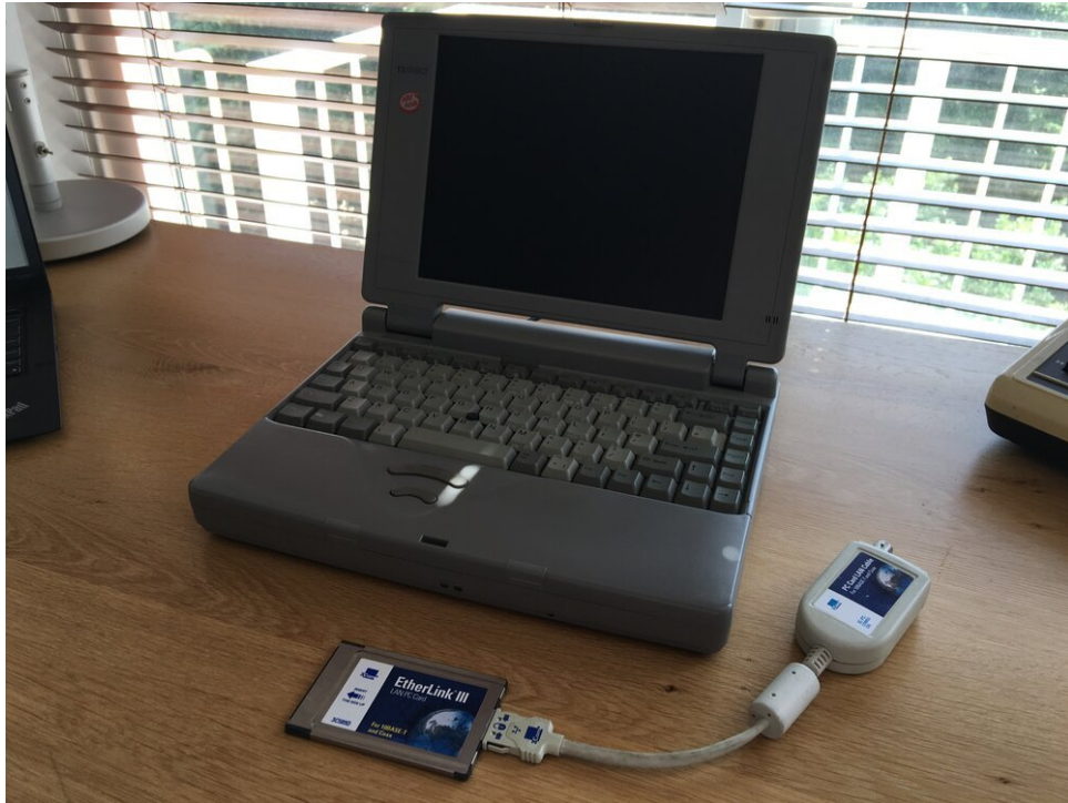
Toshiba T2130CT laptop with a 75Mhz Intel 486 processor and a whopping 16MB RAM (that is megabytes!)
