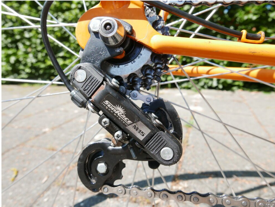
The rear derailleur was rusty and not original to this bike
