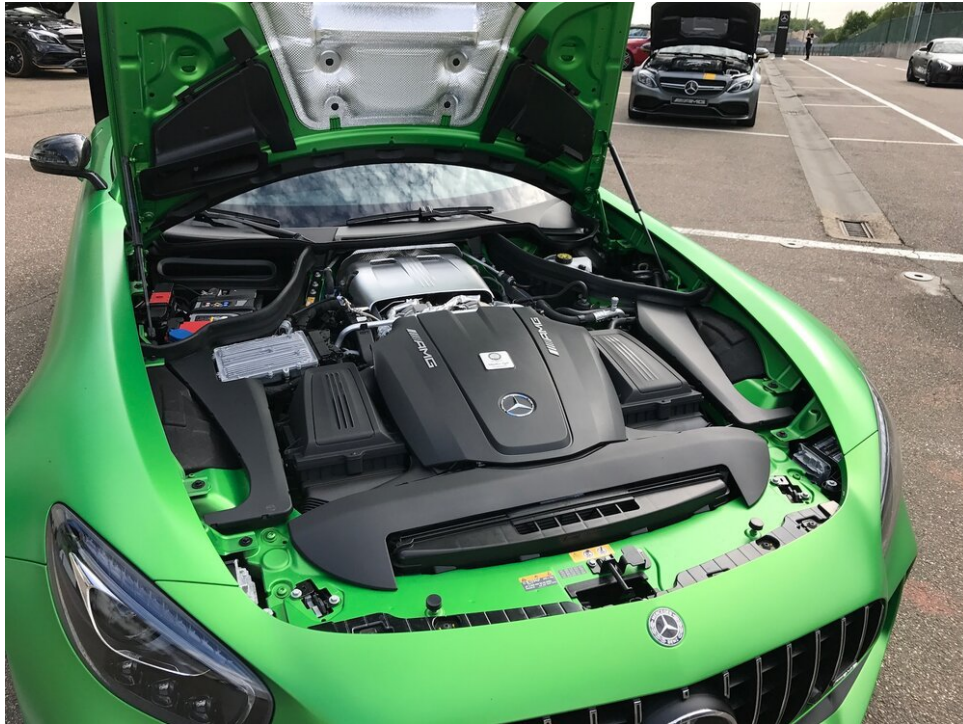
4.0L V8 Twin turbo AMG engine
