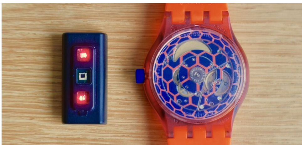
On the bottom you can see the two red LED's and the PPG sensor. Just like the Swatch Sistem51 movement this is hidden when worn on wrist
