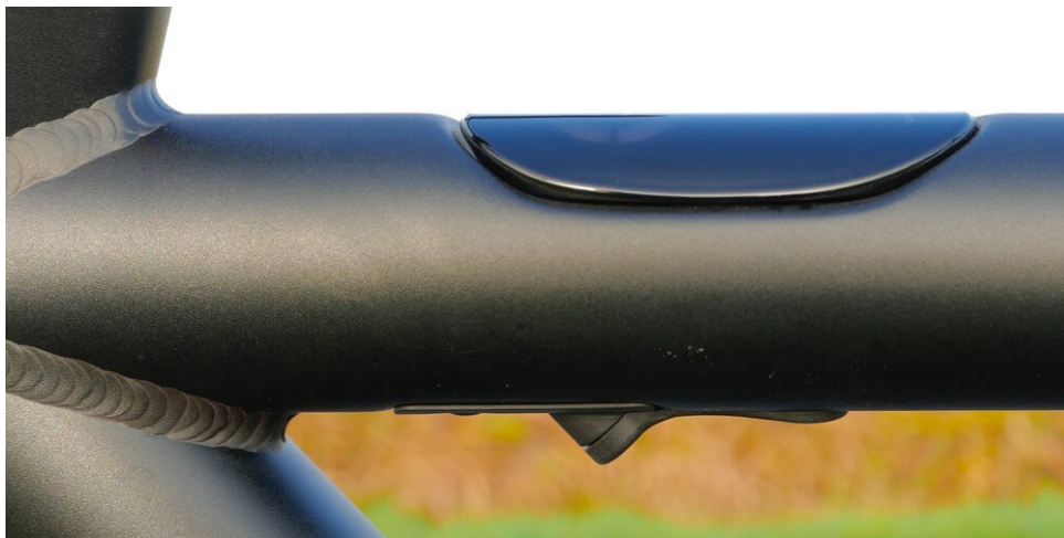
Dashboard and charging connector are integrated into the frame
