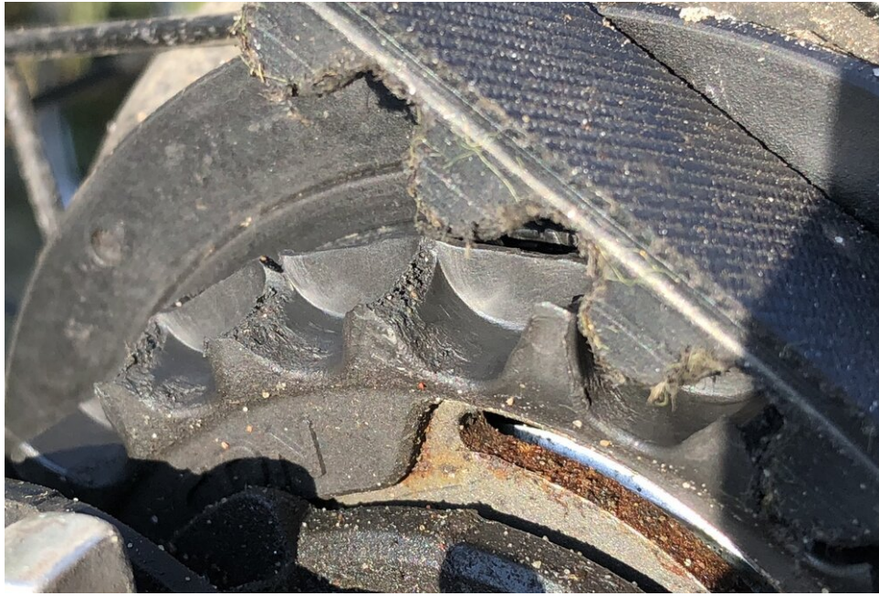
Gates Carbon Drive rear sprocket showing excessive wear after just 1800KM
