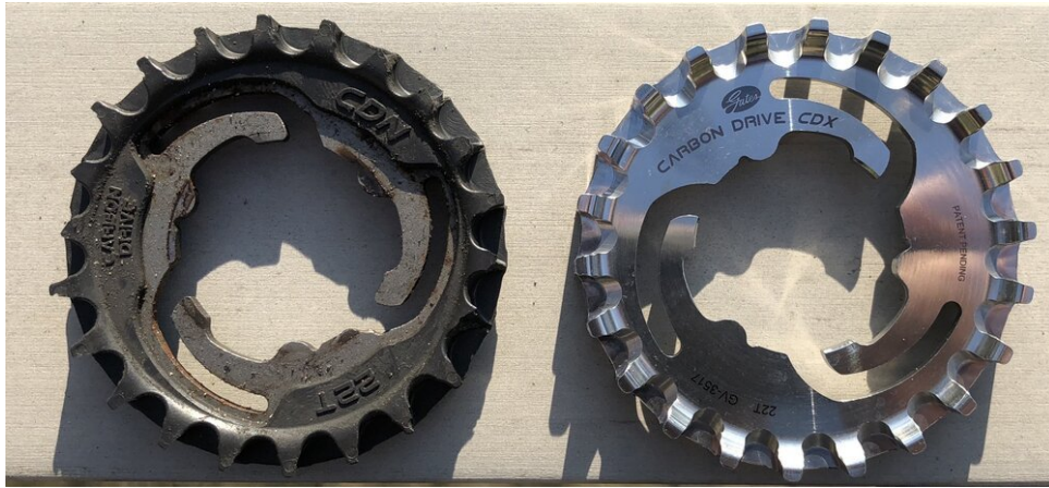
Left the plastic CDN sprocket - if you look closely you'll notice the missing teeth, right the shiny stainless steel CDX sprocket
