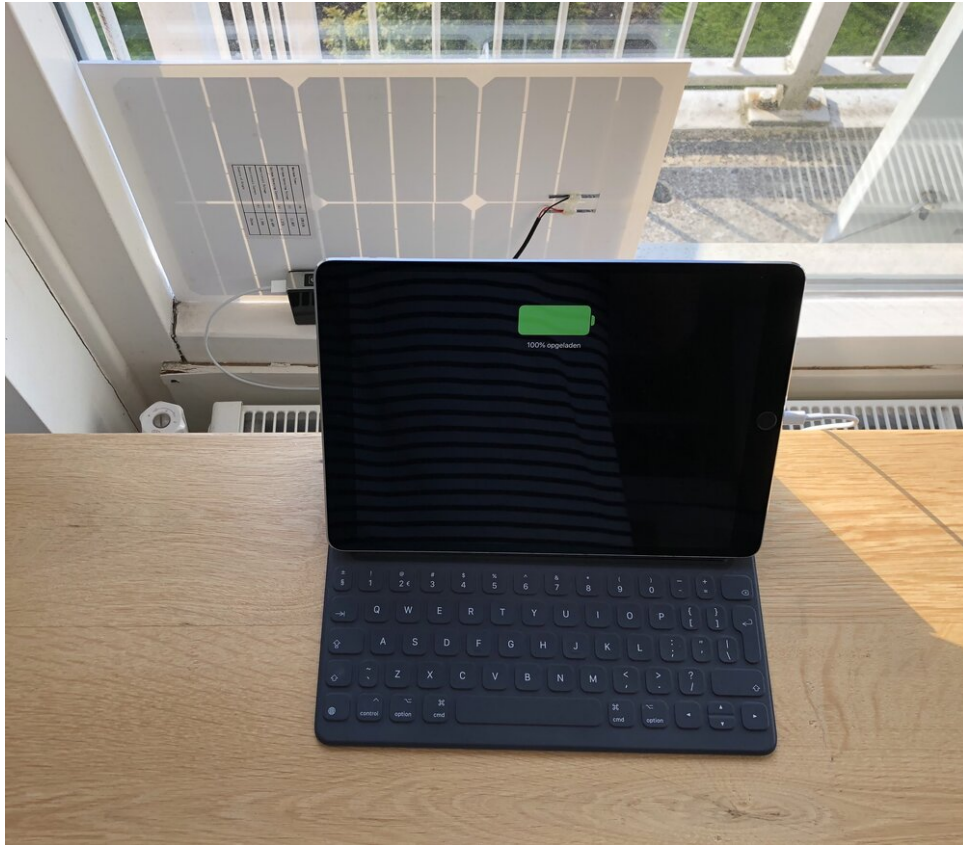
Placed behind glass the panel works, but its performance is not optimal
