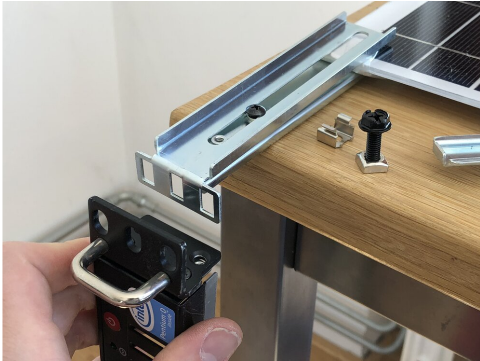
Once the front of a server, now part of the solar panel mounting fixture
