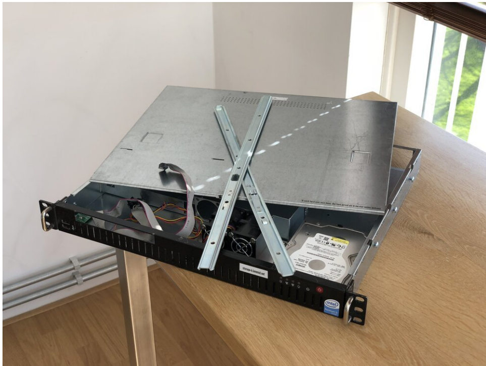
Rack mounted server chassis (1U), with rail kit
