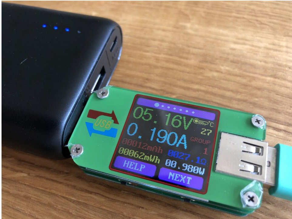
Measuring energy usage with an in-line USB power monitor
