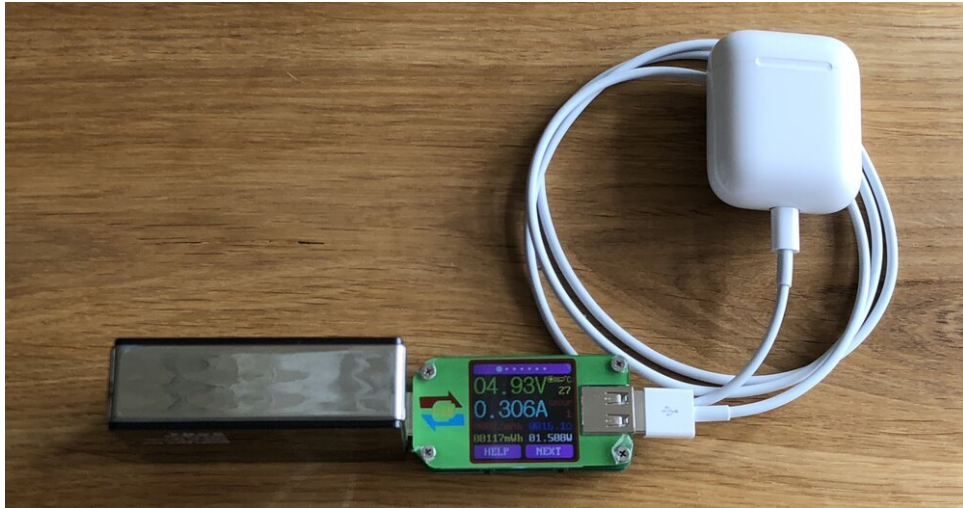
Charging AirPods using solar energy - note the higher amperes compared to the Biostrap
