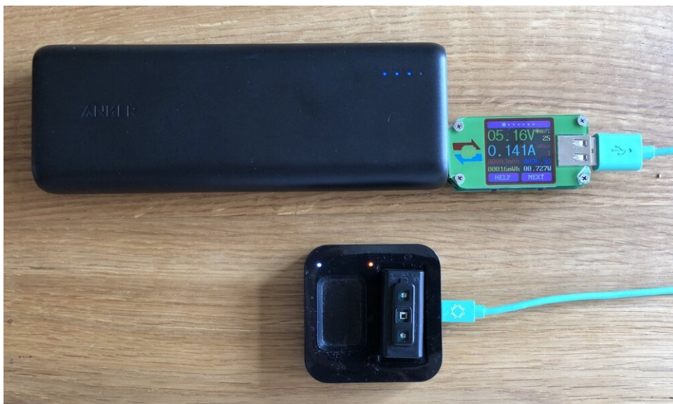
Charging Biostrap using solar energy from the Anker power bank
