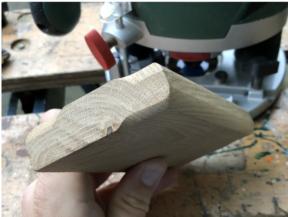
Rounding edges of the piece of wood
