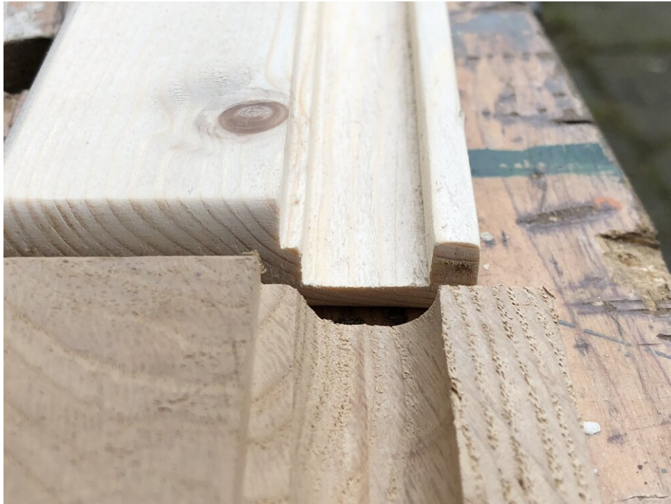
Comparing routing profile of prototype with final version
