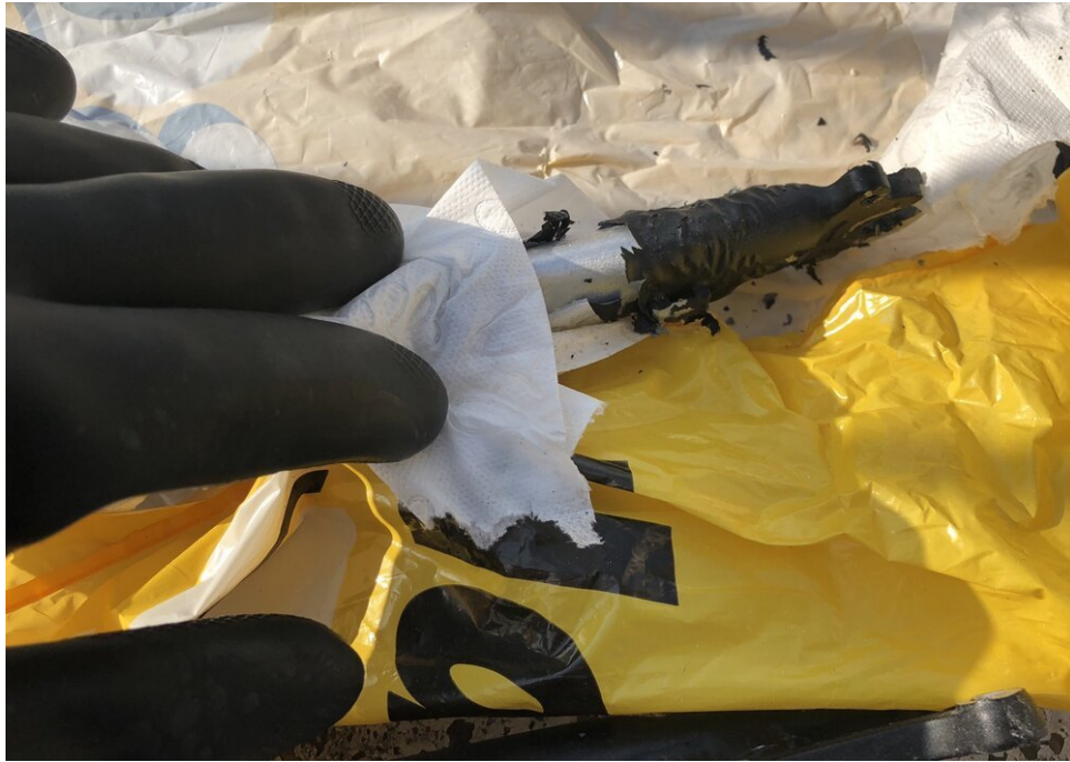
Flocks of paint falling of my bike frame, uncovering the raw aluminium
