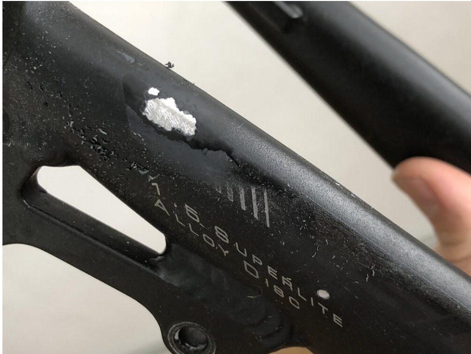
Testing the chemical solution to remove paint from my front fork - it works!
