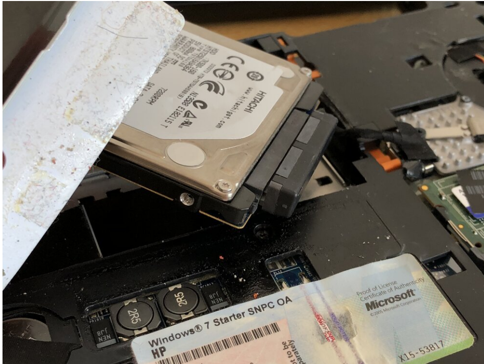
Installing the disk in the laptop
