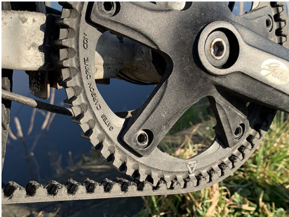
Gates CDN front sprocket and CDN belt are in good shape after 7800KM (they are original to my bike, which is about 14 months old)
