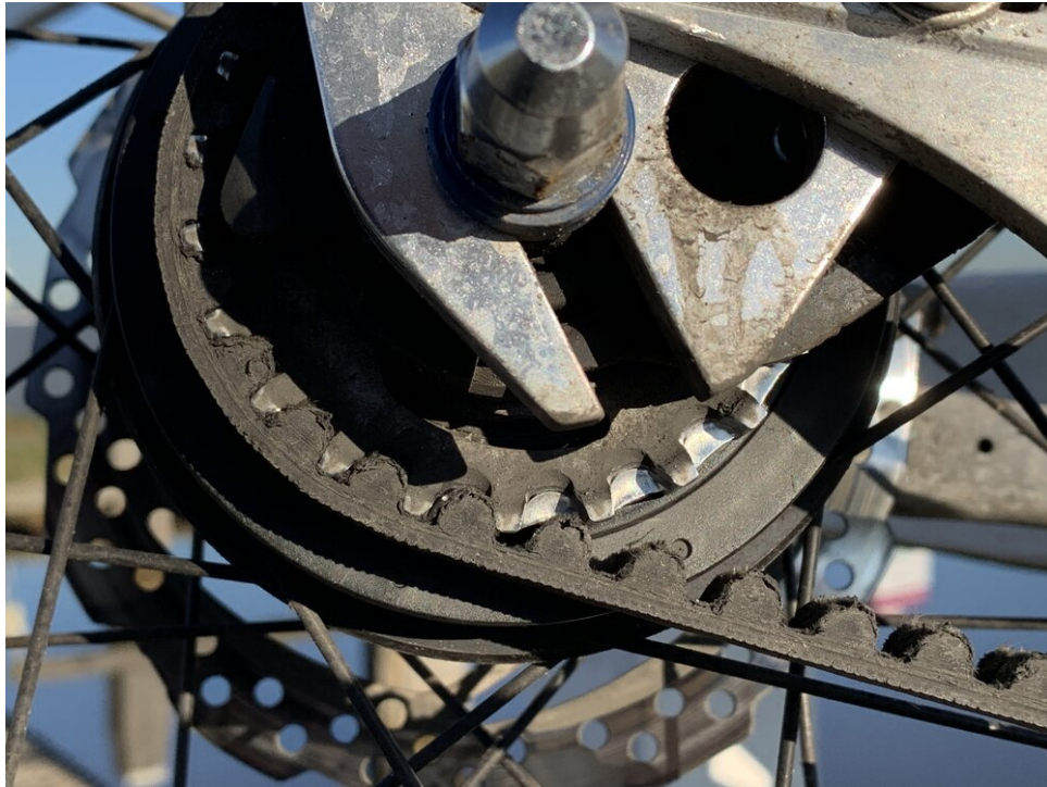
Gates Carbon Drive CDX rear sprocket after 6000KM / 12 months, a little dusty but still fine!
