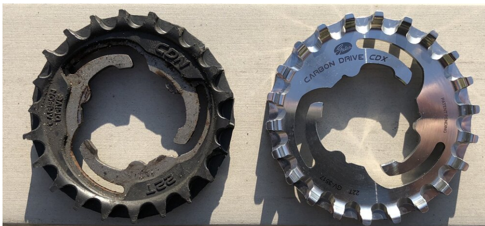
Faulty Gates Carbon Drive CDN rear sprocket left, shiny and stronger CDX sprocket right.
