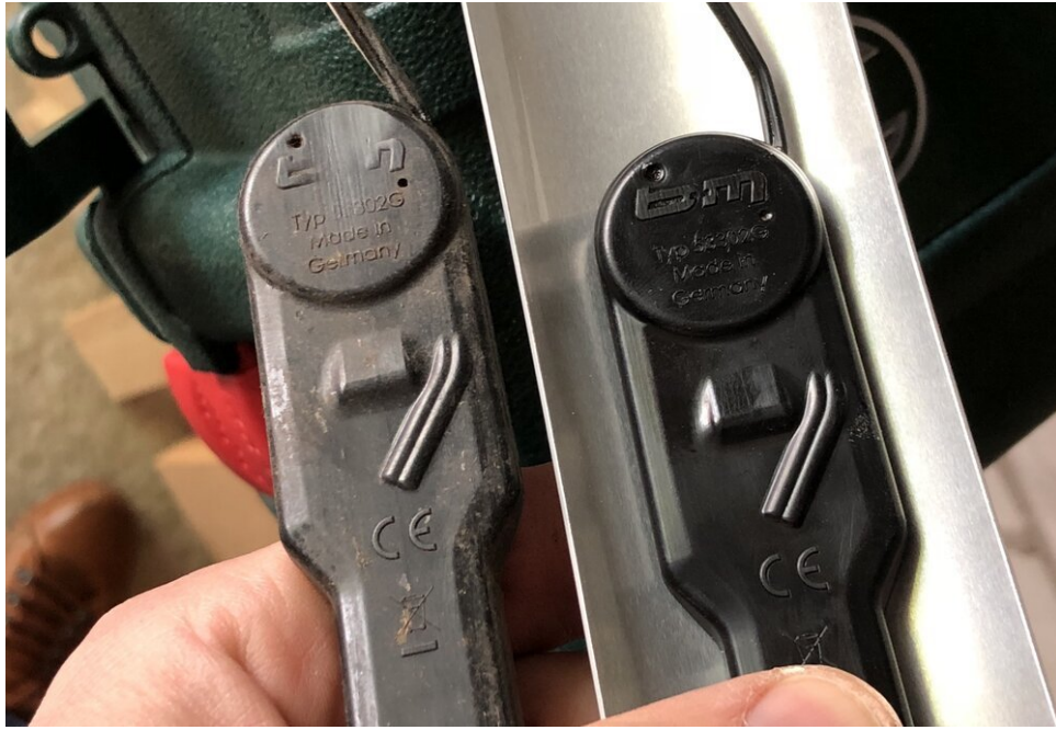
Busch und Müller rear light mounted inside the rear fender, showing signs of wear caused by the spray of dirty water from the rear tire
