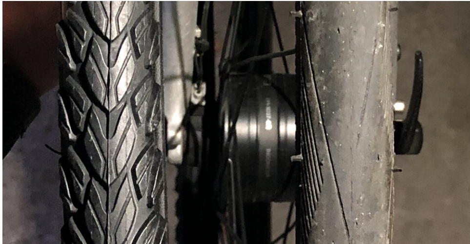
Differences in tire profile between Schwalbe Marathon Plus Tour (left) and Schwalbe Durano (right)
