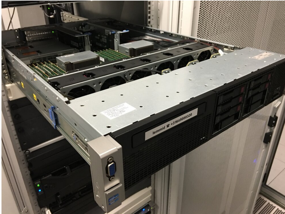
A typical server in the datacenter, a physical machine that can host apps, webshops and websites
