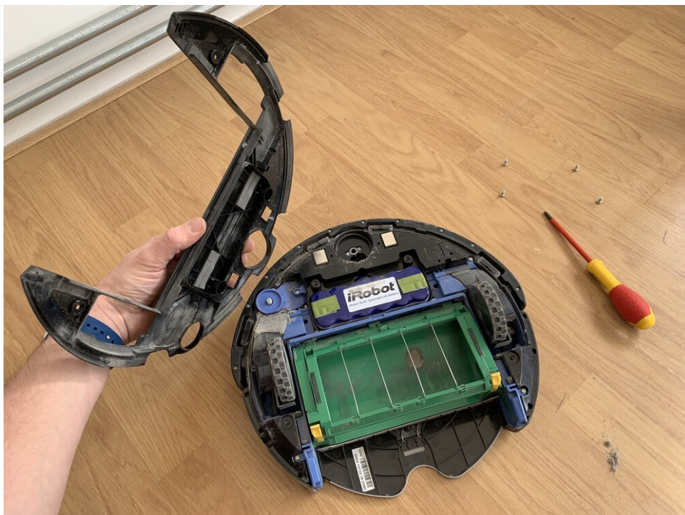
iRobot Roomba bottom cover removed
