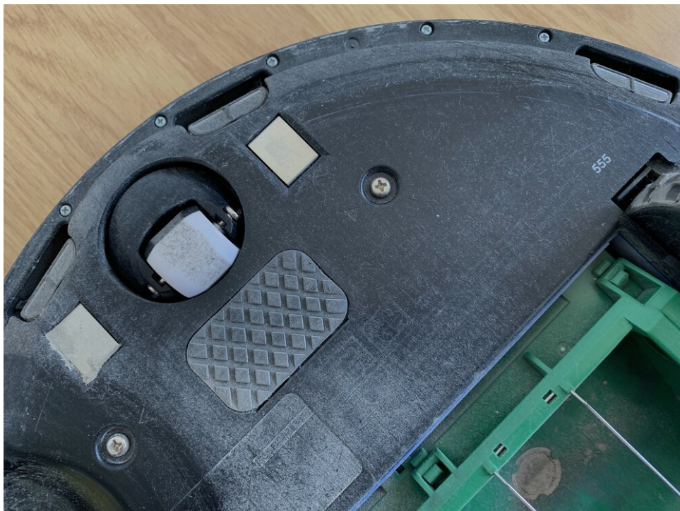
Clean "the eyes" of the Robot, the the sensor windows near the edge
