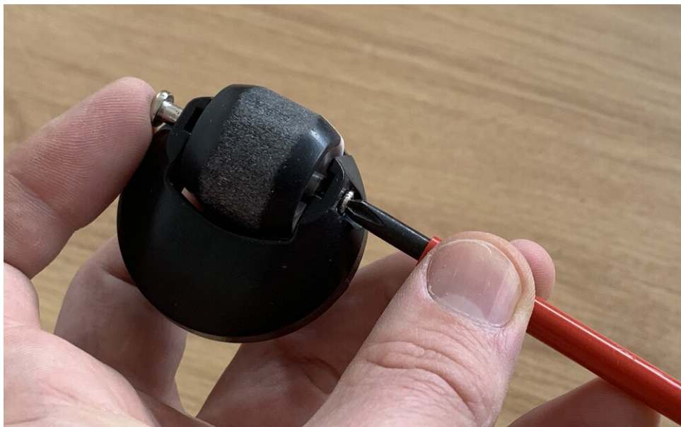
Front wheel replacement with a screw fixture
