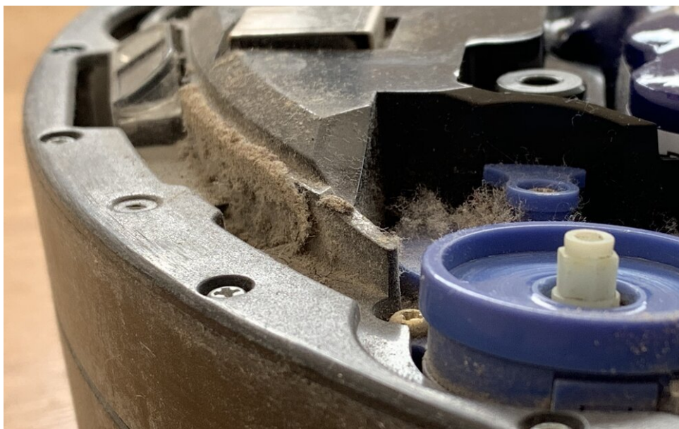
Remove dust around corners and edges
