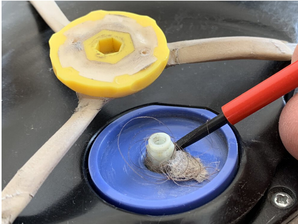
Remove dirt from the axle
