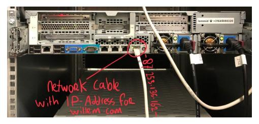
The Domain Name System (DNS) links domain names to IP-addresses, which in turn are routed through cables. You're reading this - seriously! - through the cable connected to the server shown on this photo!
