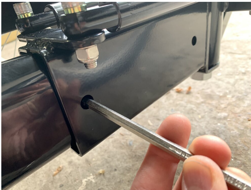
Using a hex key to nudge the filler plate into position, freeing up the bolt hole
