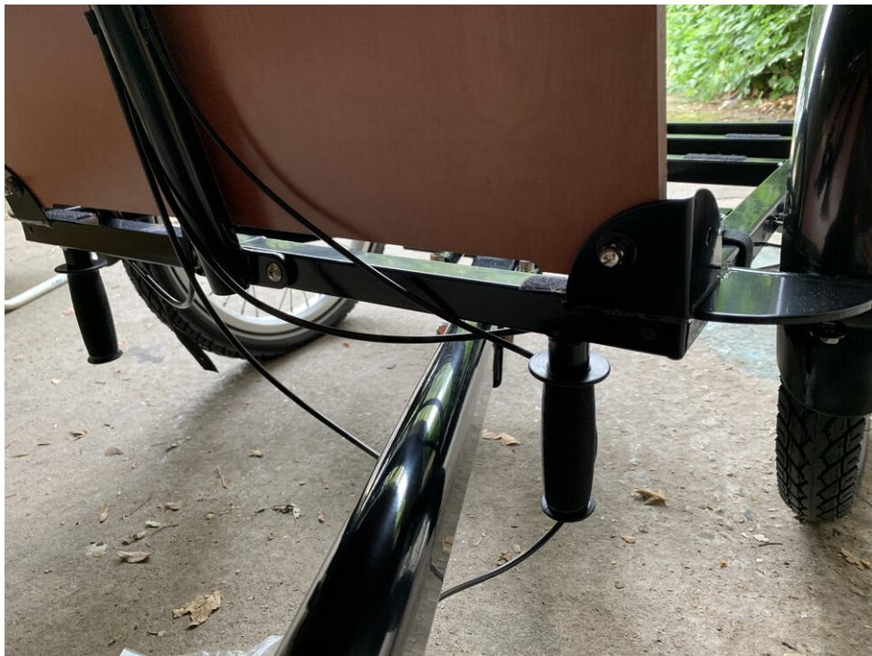
Make sure to test the swinging of the cargo box once you have fixed your cables
