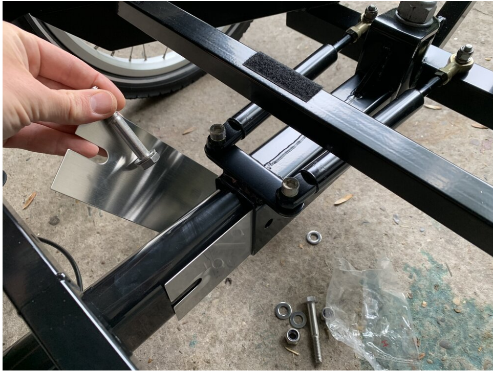
Using filler plates to make up for Chinese Precision
