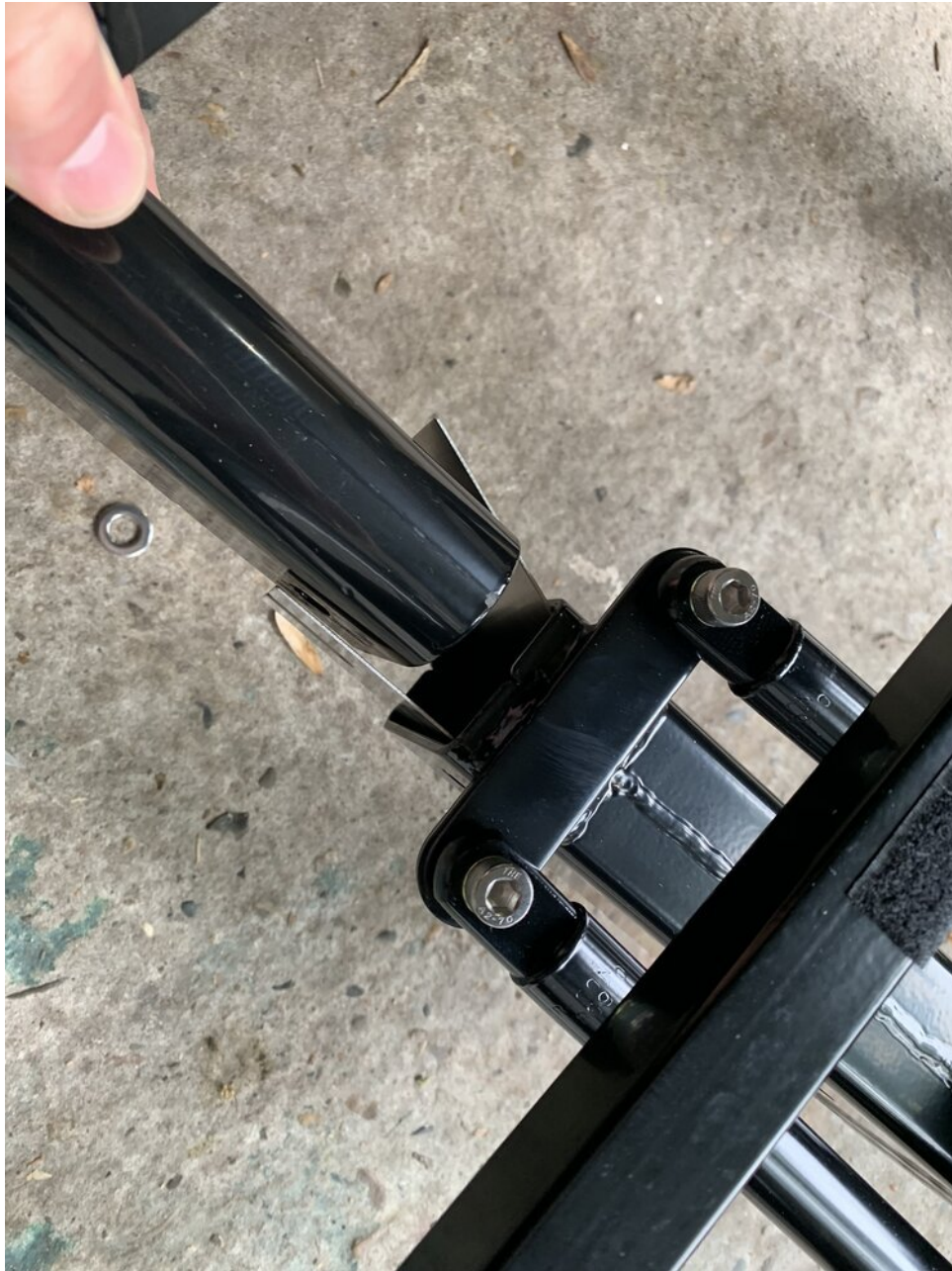
Squeezing in the filler plates while joining the rear and front frames
