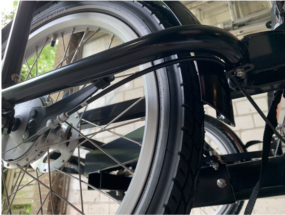
Clean cable management: I repurposed the fenders bolt to fixate the brake cable
