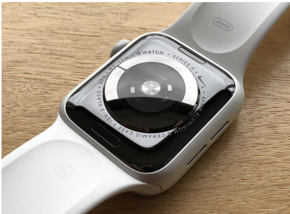
Apple Watch has an optical heart rate sensor, clearly visible in the middle of the underside
