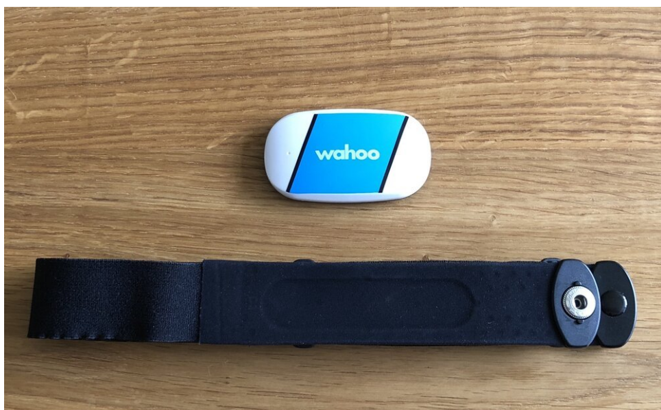
Conductive pads in the chest strap work in a similar way as the heart rate monitor in hospitals
