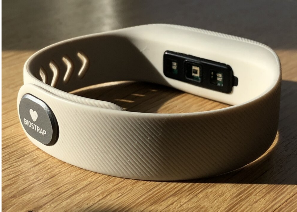
Biostrap features an optical sensor, located at the center, right between two LED's
