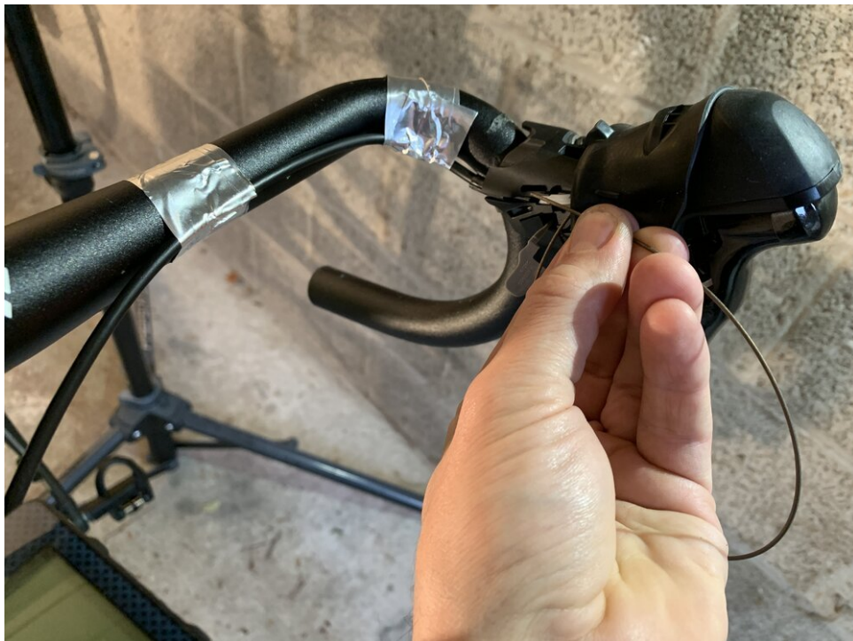
Installing cables on the handle bar and handles
