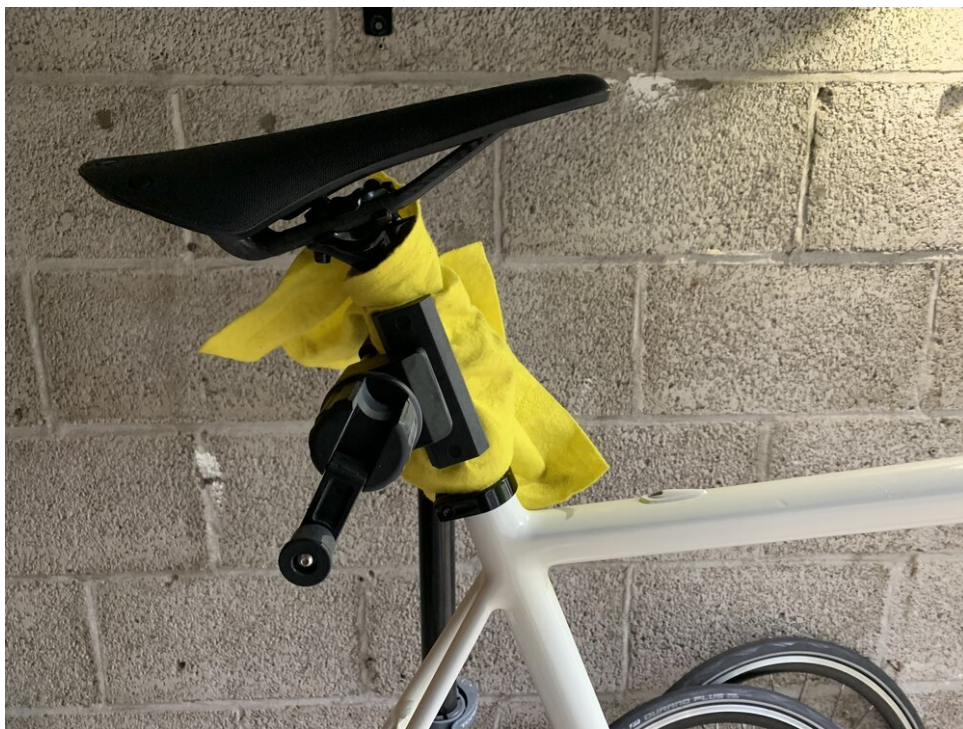
The seat post tube is a good place to fix your bike in the work stand
