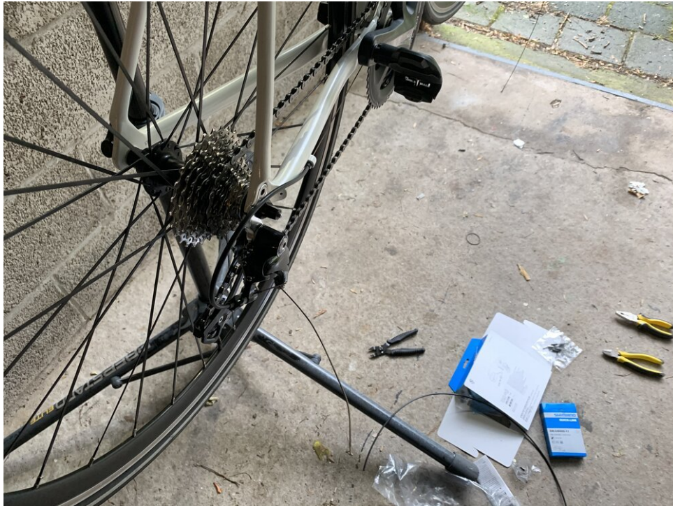
Connecting the cables to the derailleurs
