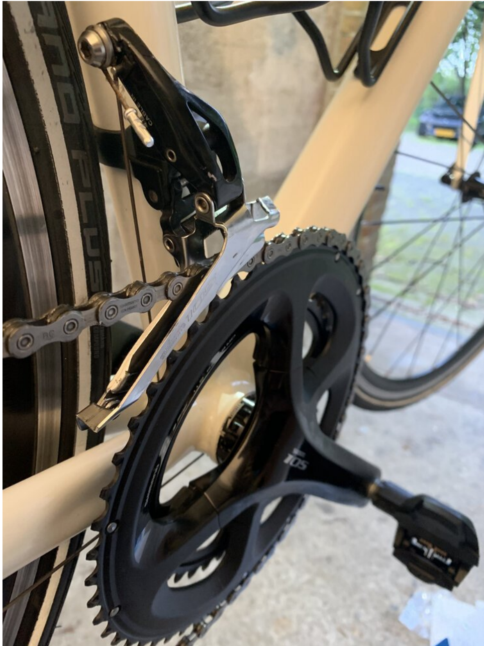
Front derailleur connected with the shifter cable
