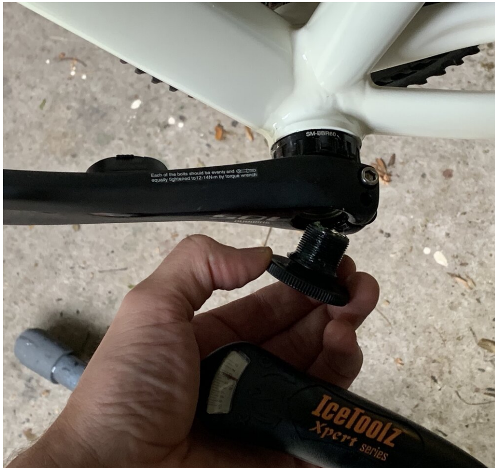
Installing the crank using a torque wrench and crank tool - note the written instructions on the crank
