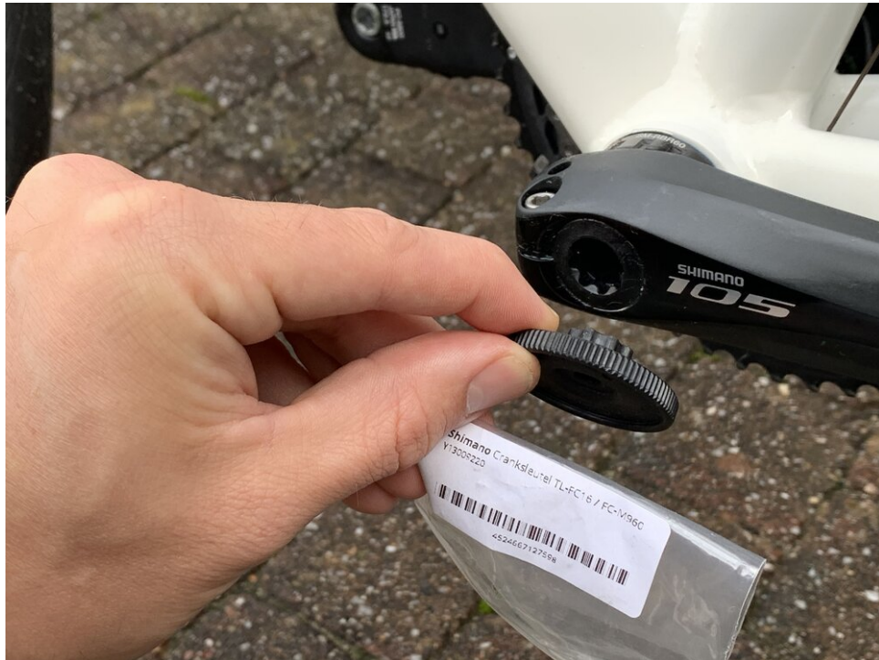
Use a crank tool to remove the crank (Shimano TL-FC16 / FC-M960)
