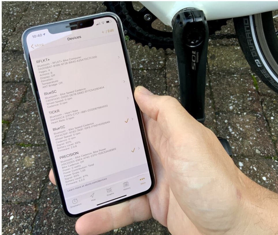
Connecting the 4iiii Precision Powermeter to the Cyclemeter app
