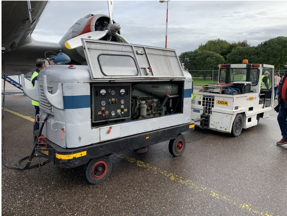
Electrical generator, powered by a German built Deutz diesel engine, used to start the R-1830 engines
