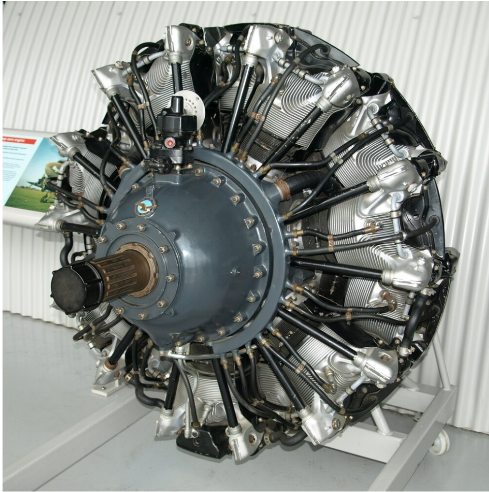
Pratt & Whitney R-1830 Twin Wasp radial aero engine on display at the Imperial War Museum Duxford (photo: Nimbus227)
