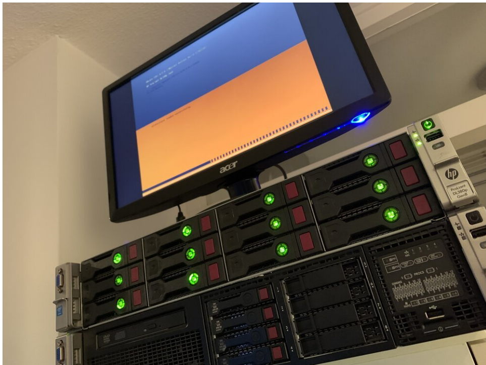
HPE ProLiant DL380p server powered on, green lights indicate the drives are working, monitor is connected and showing the boot process
