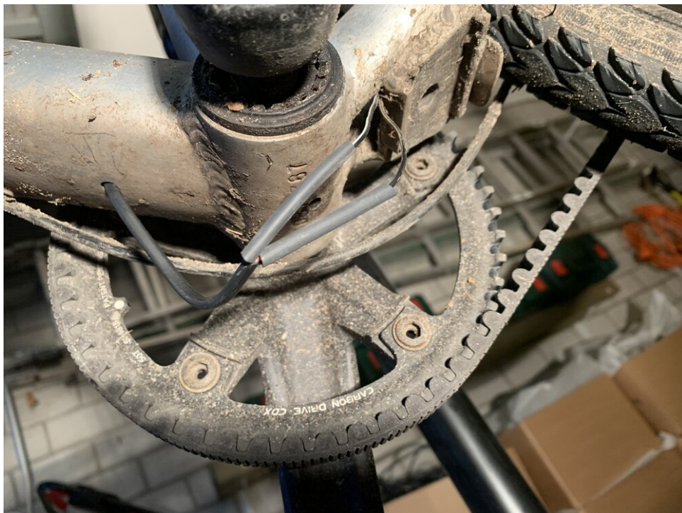
Connecting the rear light to the head light, protecting the joint with shrink wraps
