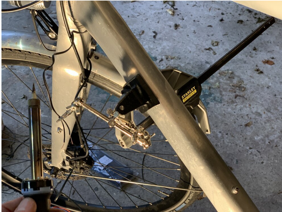
Soldering the existing cables on my bike required a little creativity using clamps
