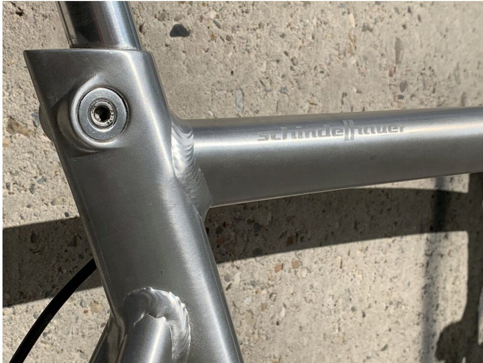
The seatpost clamp is integrated in the minimal AL6061-T6 aluminium, triple butted aero tubing frame
