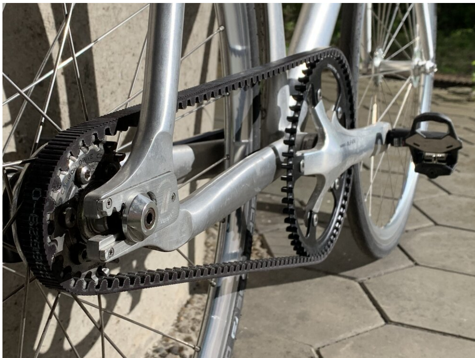
Without the conventional derailleurs the drive train is rather straightforward (60T/22T gear ratio)
