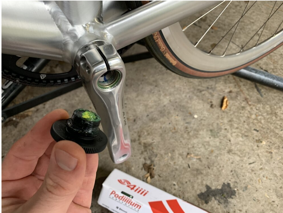
Removing the Alfine, Hollowtech II crank
