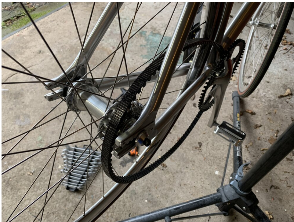
Loosen the rear axle to create just enough clearance to take the belt from the sprockets
