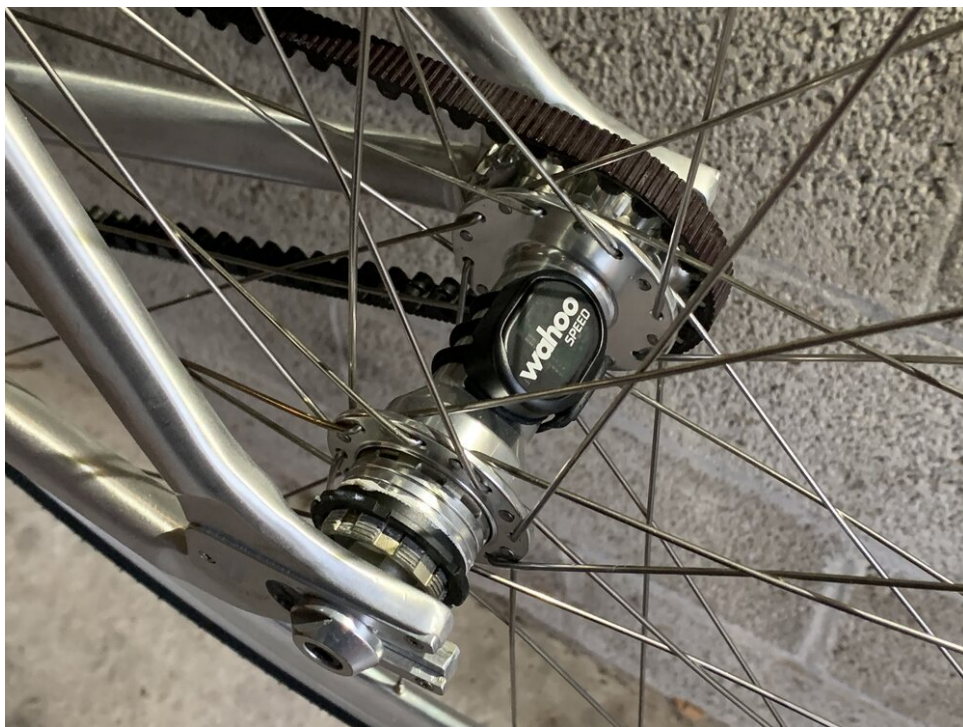
The Wahoo Speed sensor installed on the flip-flop rear hub
