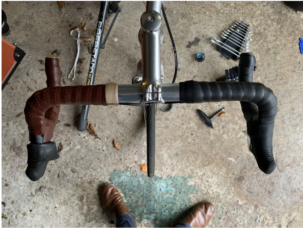
Replacing the brown leather with black rubber bar tape (from Brooks)
