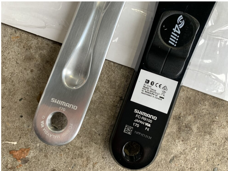
The Shimano FC-R9100 Dura Ace power meter by 4iiii fits perfectly
