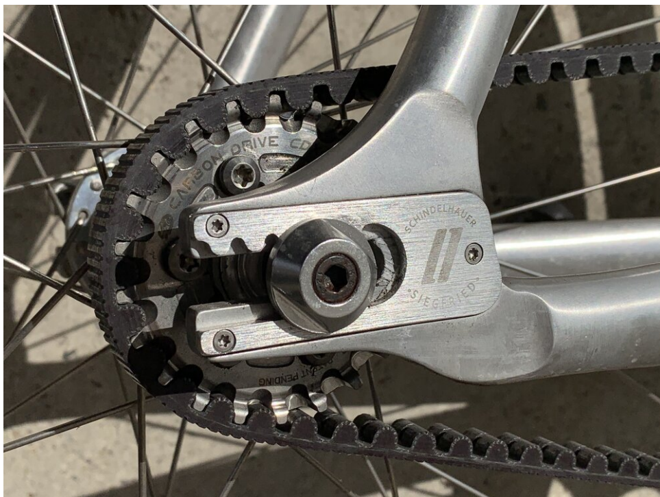
The rear wheel is fixed using a 'crocodile' belt tensioning system
