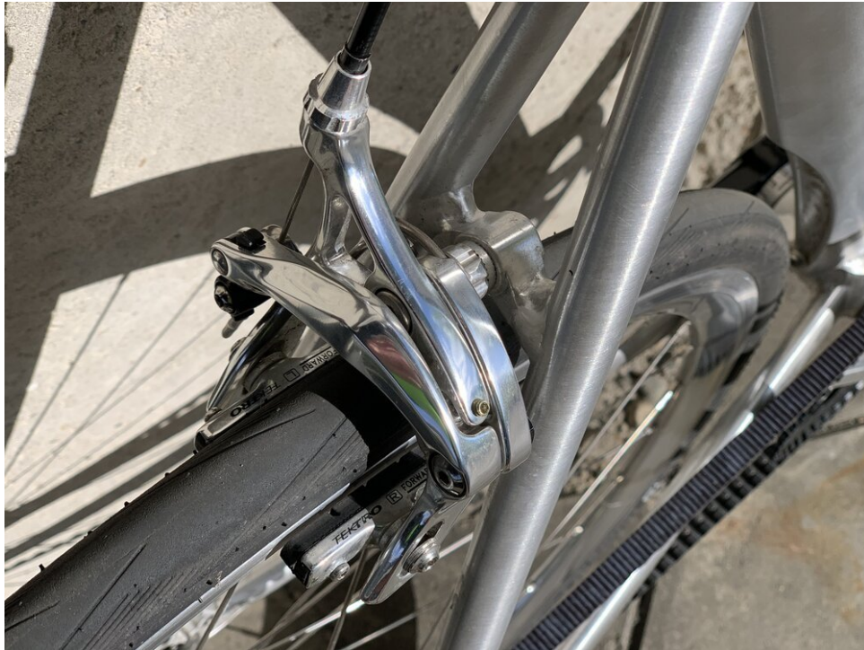
Siegfried Road features simple, yet very functional Tektro R539 / TRP - RRL brakes
