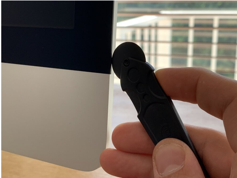
Using a special roller to cut the iMac open
