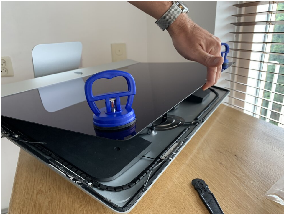
Be careful when lifting the glass, there are cables connecting the panel to the logic board
