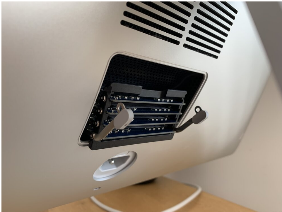
The RAM hatch pops open using the secret button inside the power connector
