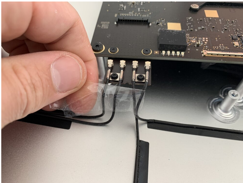
Removing the antenna cables, remember their order using a piece of tape
