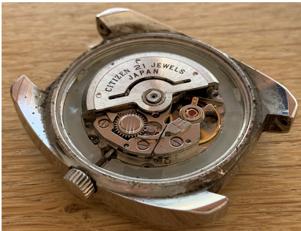
There is a rotor that winds the watch when it is moved (on the wrist), a clever system that negates the need for batteries
