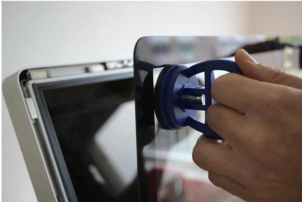
Removing the glass panel using suction caps
