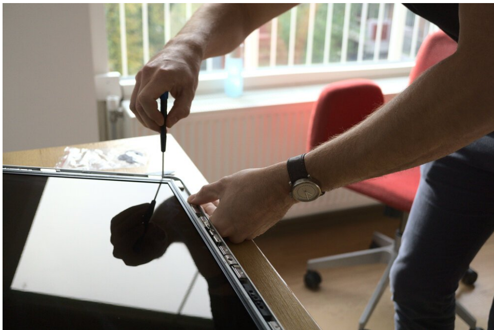
The display is fixed using Torx screws - it can be a little tricky to remove the screws as the magnets easily catch them!
