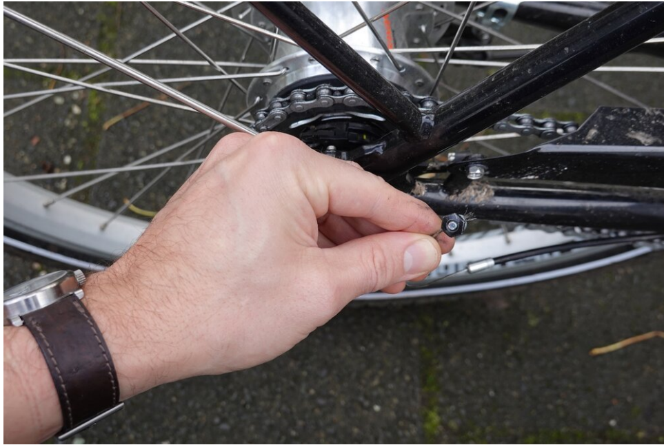
The bolt holding the gear cable pulled out of the bracket at the gear hub
