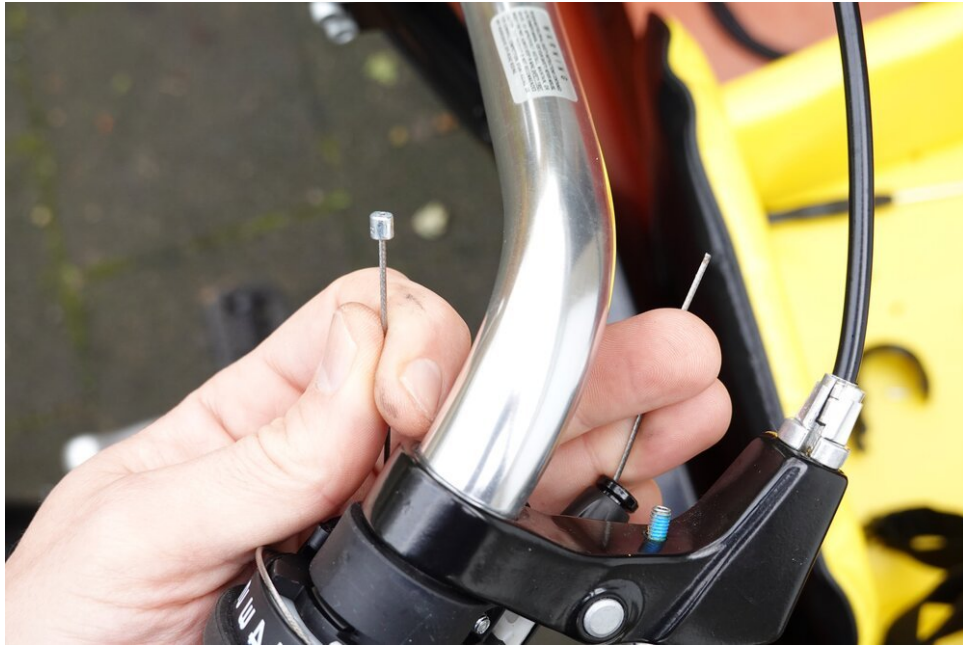
Install the new shifter cable starting from the handle bar
