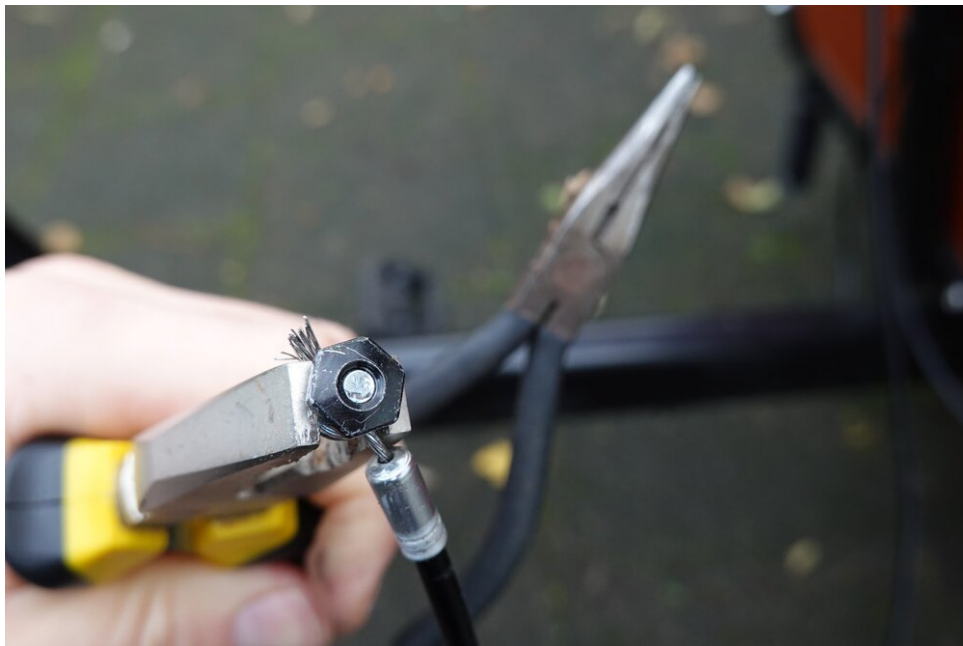
Loosening the bolt is easily done using two pliers
