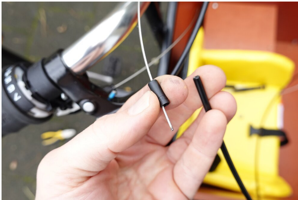
Make sure you include + install all the end caps as they prevent moisture and dirt from entering the outer cable(s)
