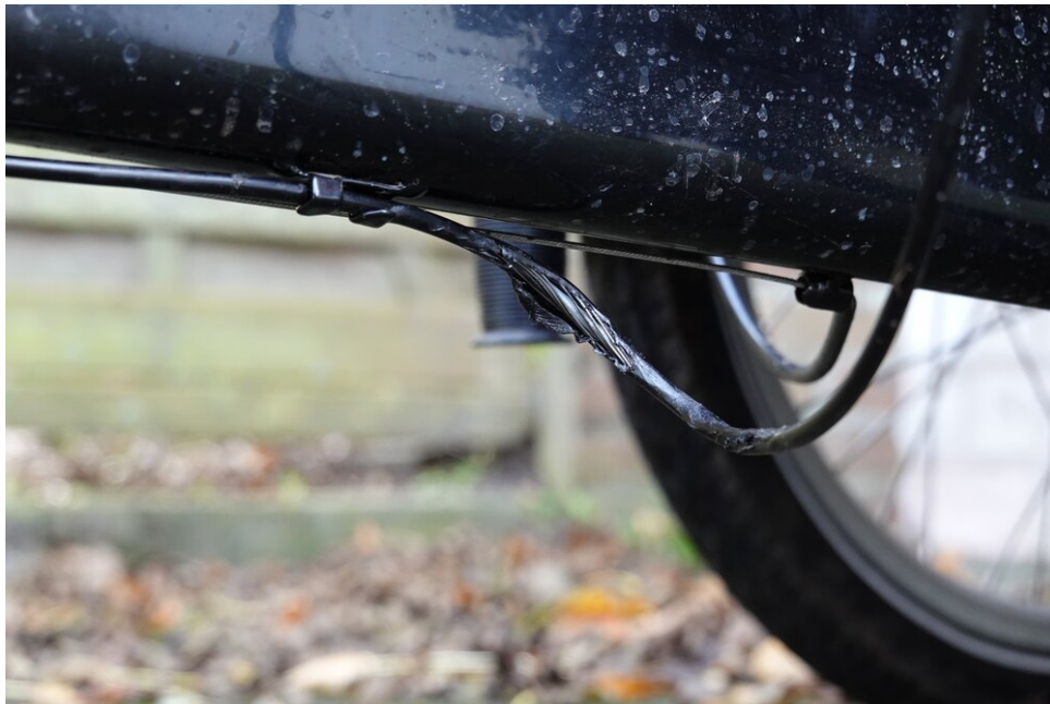
The shifter cable underneath the cargo bike was pulled apart by a branch...
