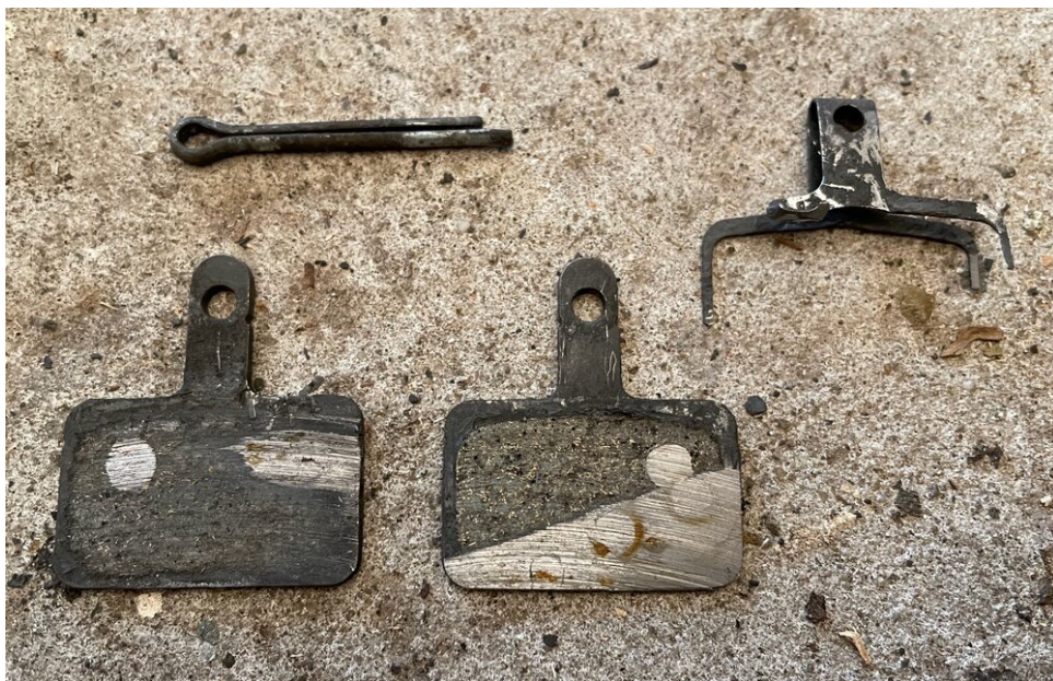
My hydraulic brake pads were worn out! Note the damaged fork in the upper right (which is supposed to keep the pads in place)
