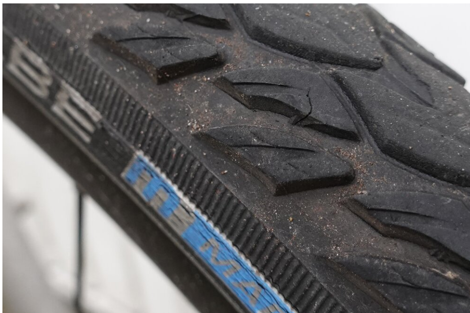
Only some signs of wear after 11.000KM - and not a single puncture!
