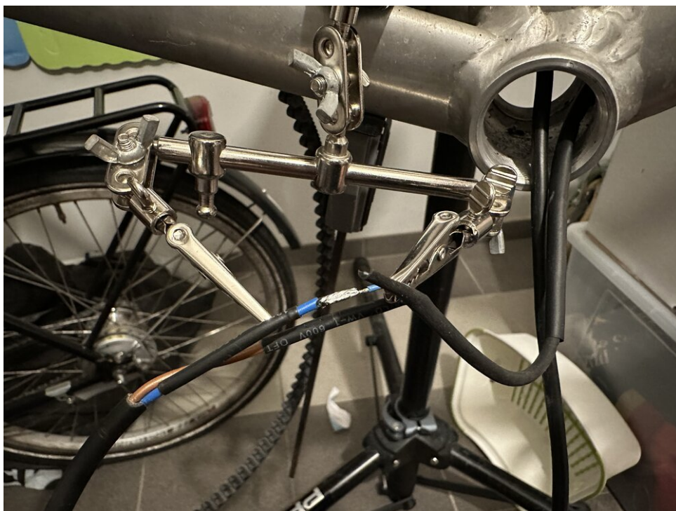
Soldering the individual leads together and shrink wrapping them
