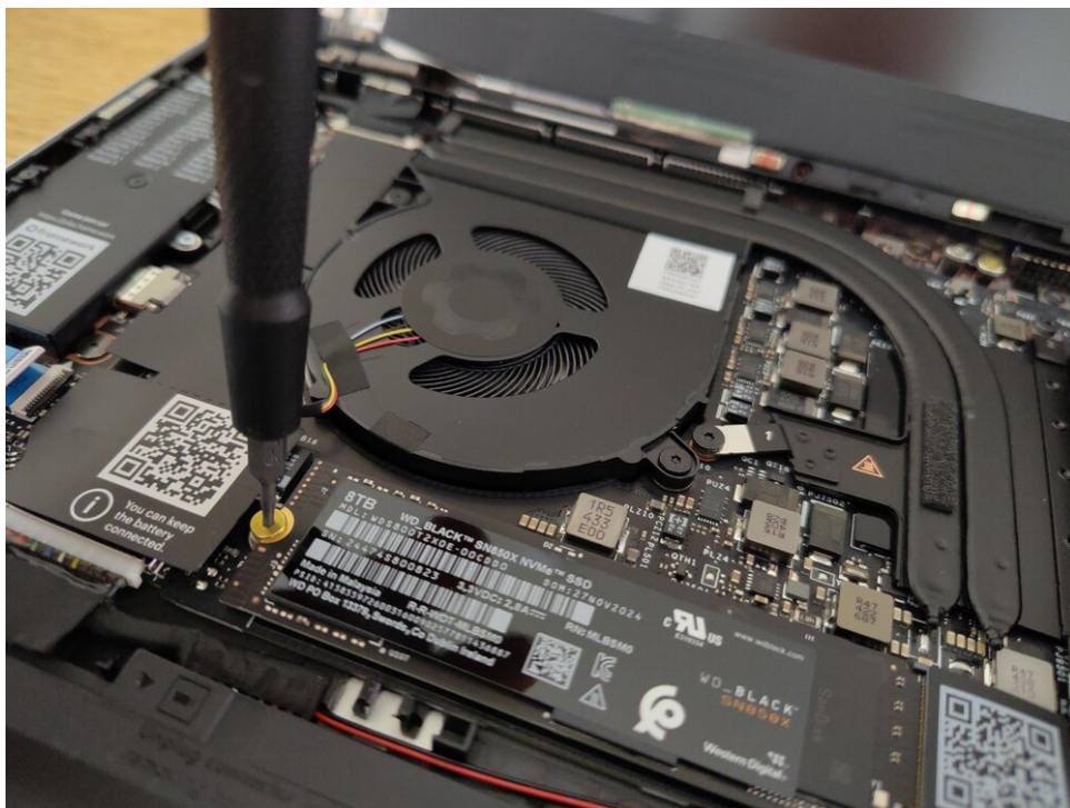
The 8TB SSD is secured with a single screw
