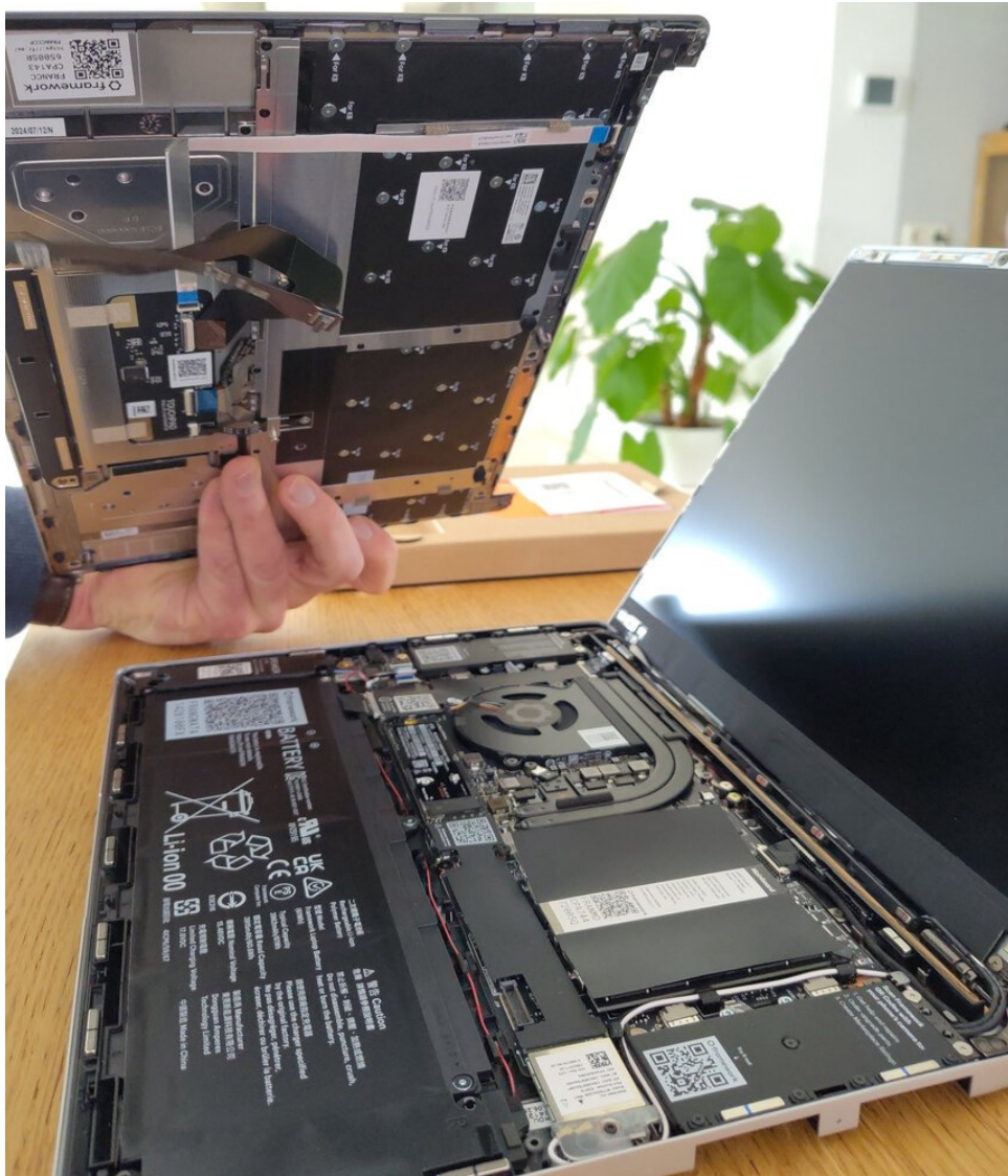
The keyboard cover snaps into position using magnets and is secured when you tighten the screws in the bottom cover
