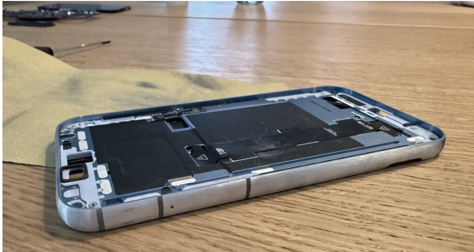
Using sanding paper to remove paint from the Fairphone
